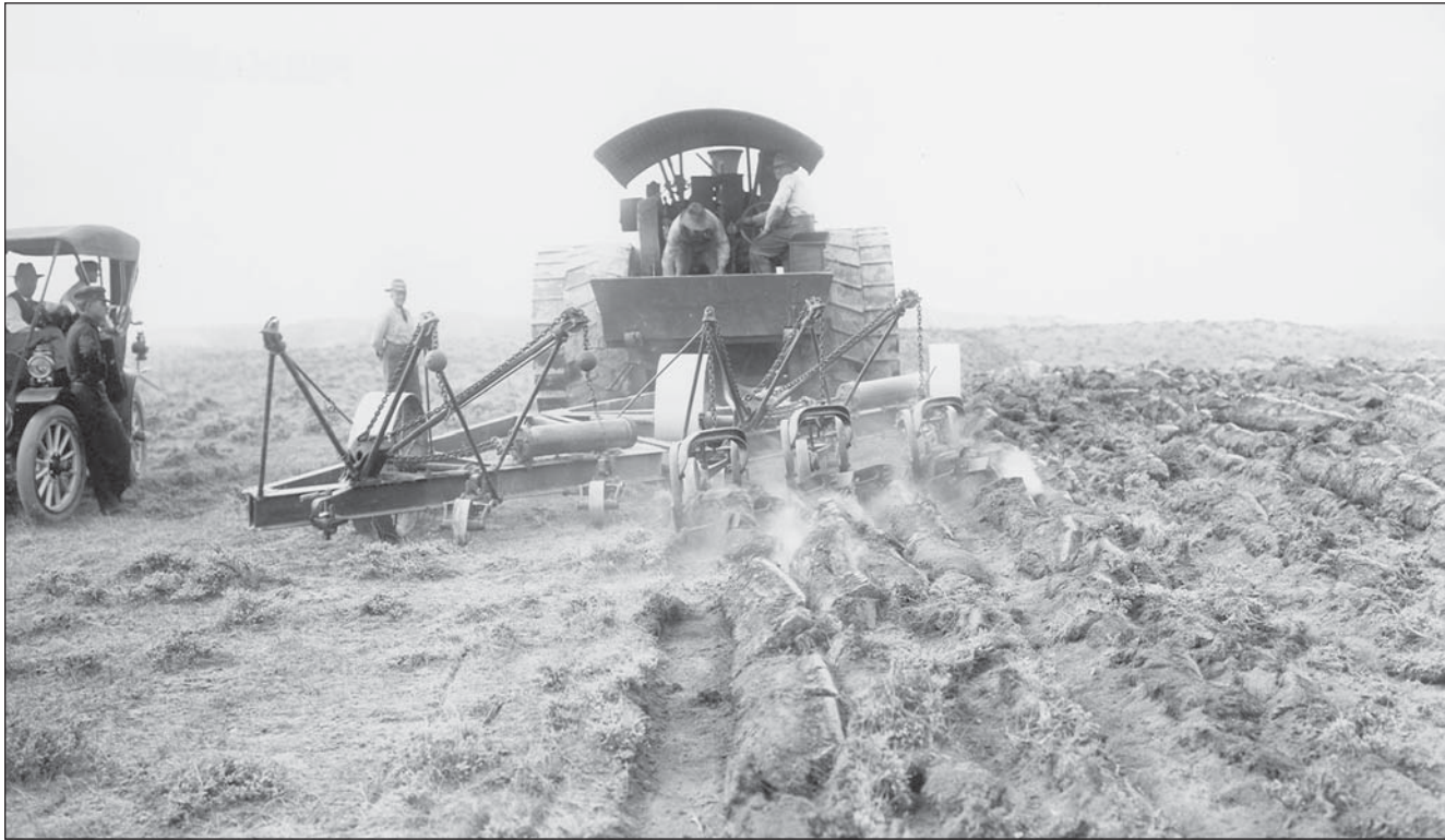
Steam plow on Unland's farm, Douglas. This steam tractor is the same device that would power threshing machines; here it is breaking sod. The huge machine required two operators on board, both visible in this photograph. Photo: J. E. Stimson Collection, Wyoming State Archives, negative 2925.
