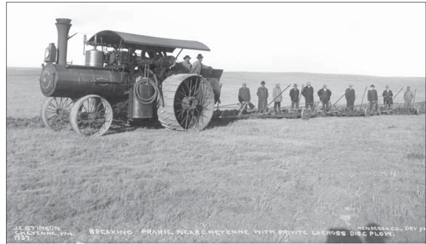
Breaking Prairie near Cheyenne with Reeves steam traction engine and LaCrosse Disc Plow. Photo: Stimson Collection, Wyoming State Archives, negative 2925.
