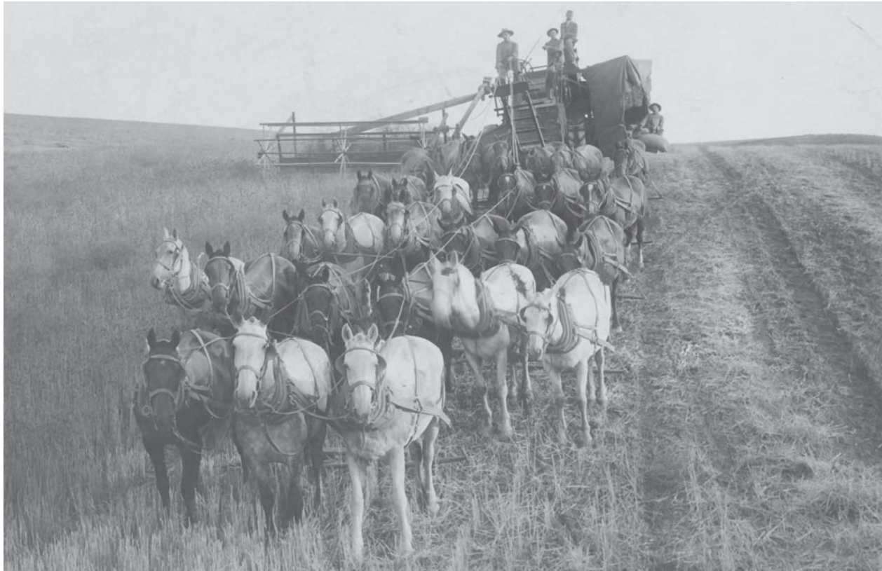
The combine was a complex industrial operation that moved through the fields, cutting and threshing the grain as it traveled. Note the bags of grain on the right side of the machine as well as the horsepower required to pull it. This harvesting operation probably was in the Eden Valley. Photo: courtesy Sweetwater County Museum, Green River.
