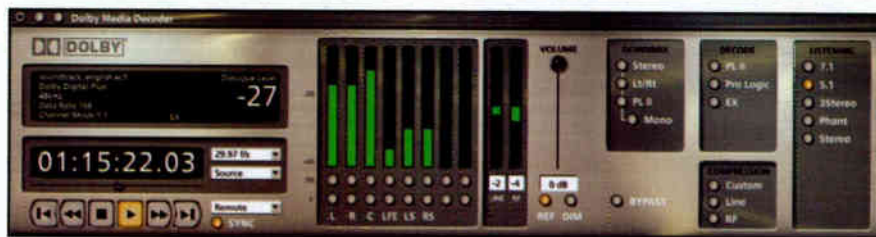
The Decoder allows decoding/monitoring of Dolby Digital Plus, Dolby Digital, TrueHD and MLP Lossless formats.
