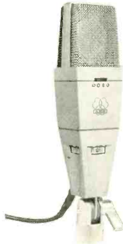
C414 (C 414C comb. with DIN plug on request.) FET Studio microphone with large condenser capsule. Pattern selector on microphone for cardioid, omnidirectional, figure of eight and hyper-cardioid. Switchable -10 db attenuator.
