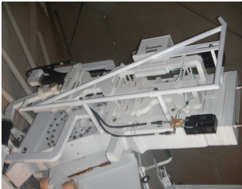
The RF Pallet, part of the Dual Polarization upgrade. This component splits the main transmitted pulse into horizontal and vertical components.
