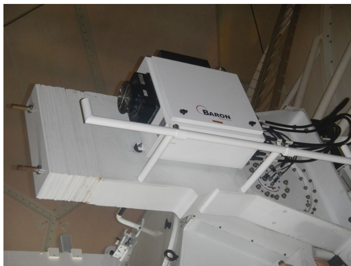
The AME, or Aerial Mounted Equipment, processes the dual polarization returns.
