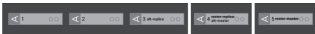
Figure 11: The roster-master and roster-replica are in minority clusters, cluster is split, p is inactive
