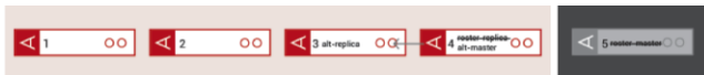
Figure 10: The roster-replica is in majority sub-cluster, promoted to master, alt replica created in node 3, cluster is split, p is active
