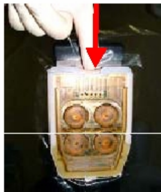
Figure 3-5 壓下消毒轉接頭釋放突片
