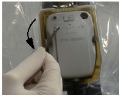
Figure 4-9 用扳手打開器械
