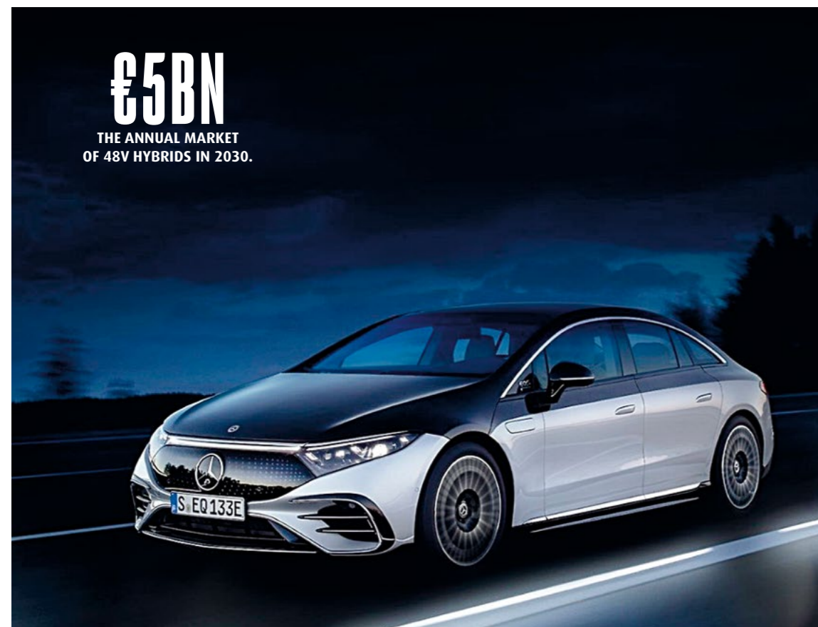
The Mercedes-Benz EQS - the flagship model in the premium automaker's electric vehicle range - is powered entirely by a Valeo Siemens eAutomotive system combining two electric motors (300kW of power at the rear and 170kW at the front), an inverter - the brain of the system - and a reducer.
