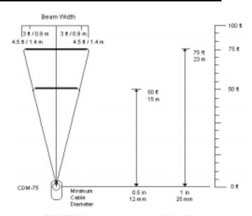
CDM-75 Measurement versus Cable Diameter
