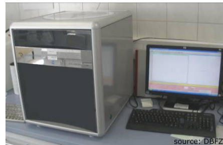
Figure 10: CHN-analyzer according to EN o 15104
