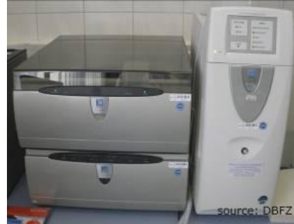
Figure 9: Analyzer for S & Cl according to EN o 15289
