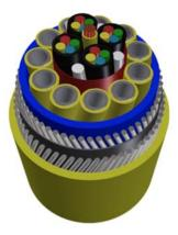
UFLEX is a special purpose program system for non-linear stress analysis of complex umbilical cross-sections.
