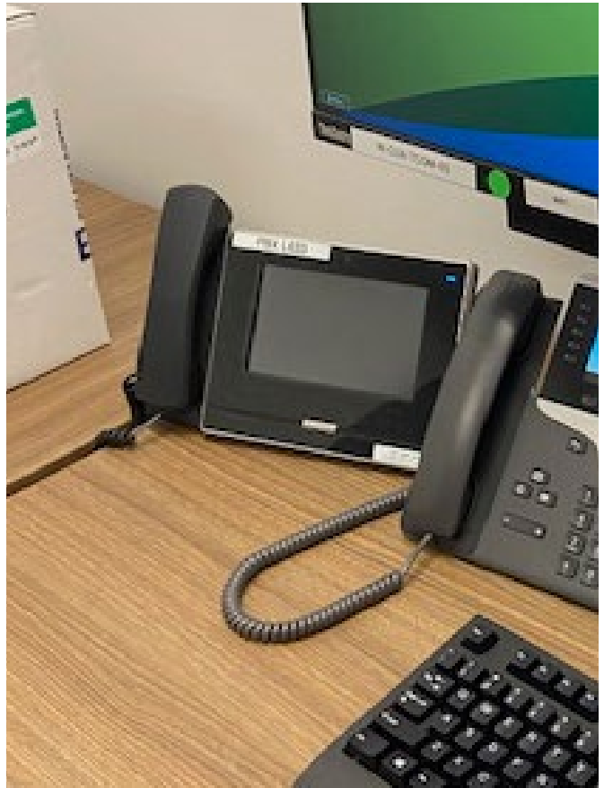
Primary calls could be transferred to another IP Video Master Station (IX-MV7-HB) , where authorized personnel at that location can determine how the call should be addressed.
