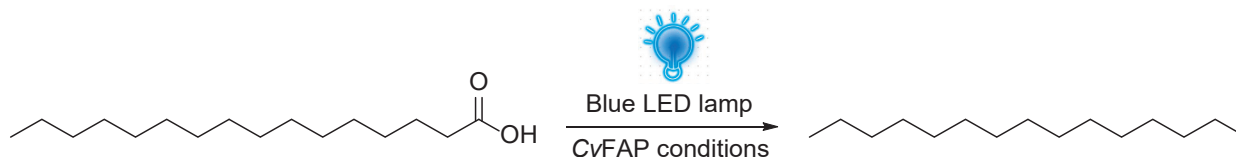
Scheme 1: Palmitic acid decarboxylation via CvFAP.
