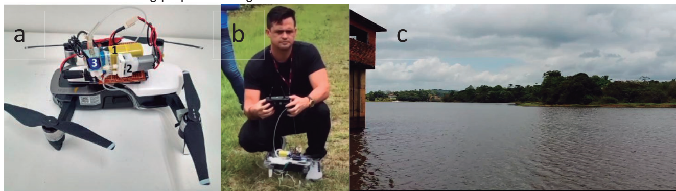
Figure 1. UAV adapted (a) for water sampling with 1 (battery), 2 (MP), 3 (SV), and UAV used to collect water and real time data transmission (b). Image of Water reservoir captured using the UAV during the in situ analysis (c).
