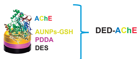
Scheme 1. Schematic representation of DES-AChE construction.
