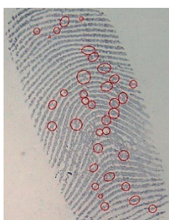
Fig. 1: Minutiae count revealed with produced powder
