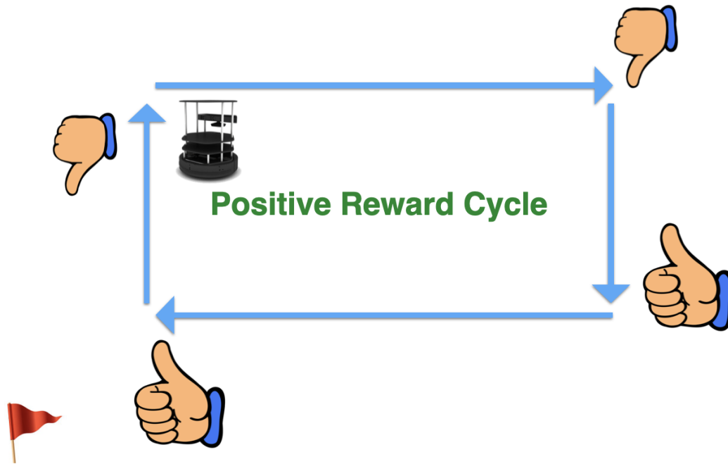
FIGURE 3.1: The goal of the task is to teach the robot to move to the red flag at the bottom left corner. The human trainer gives big positive reward when the robot moves closer to the flag, and small negative reward when it moves away, which leads to a positive reward cycle.
