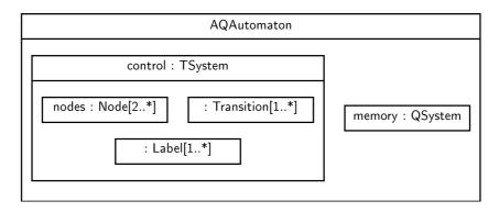
Fig. 1. Composite structure of an abstract quantum automaton
