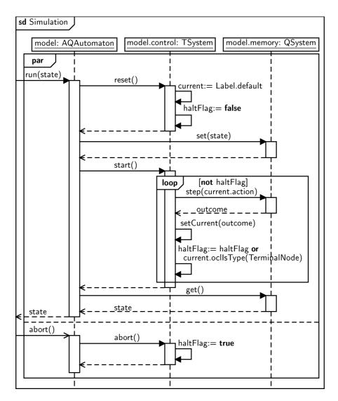
Fig. 3. Abstract quantum automaton behavioural model: interaction of components
