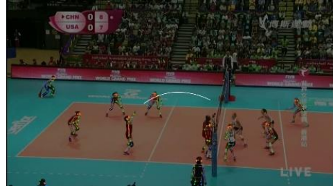
Figure 6: Example 2D application of player identification and identification of ball trajectory changes ("trigger"). Keypoints can be observed on each player's silhouette, along with the corresponding arc of the ball trajectory.
