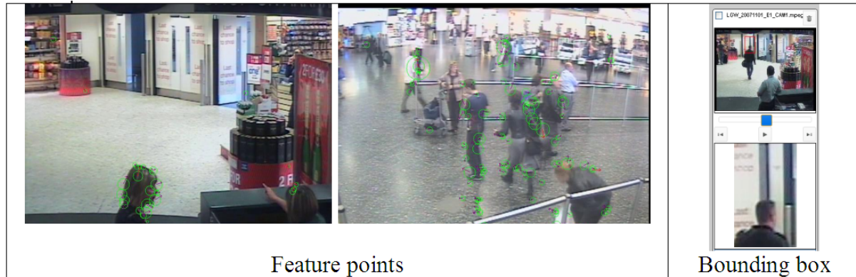
Figure 7. Extracted meta-data, such as rectangles, points, and vectors detected by the detection algorithm, can be used by VAP Event Browser interface to make visual processing more efficient through the use overlaid graphical annotations and extracted regions of interests.
