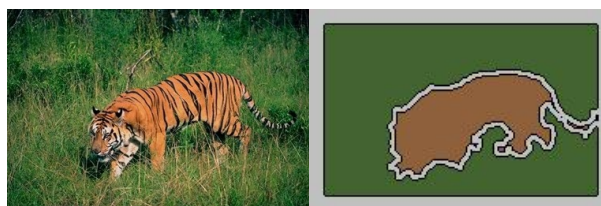
Figure 2.3: The role of segmentation in recognition. The average color of pixels in each segment determines the displayed color.
