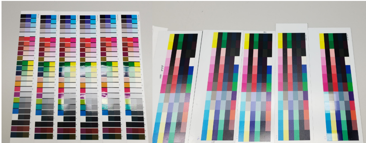
Figure 1: Fogra MediaWedge CMYK v3 printed in 2D print on a semi-matte paper (left). The applied tone values of varnish are: (from left to right) 0%, 20%, 40%, 60%, 80%, and 100%. On the right is the Fogra MediaWedge CMYK v3 printed in 2.5D print with different print settings and types of varnishes categorised as 1-1, 2-1, 2-2, 1-3 and 2-3
