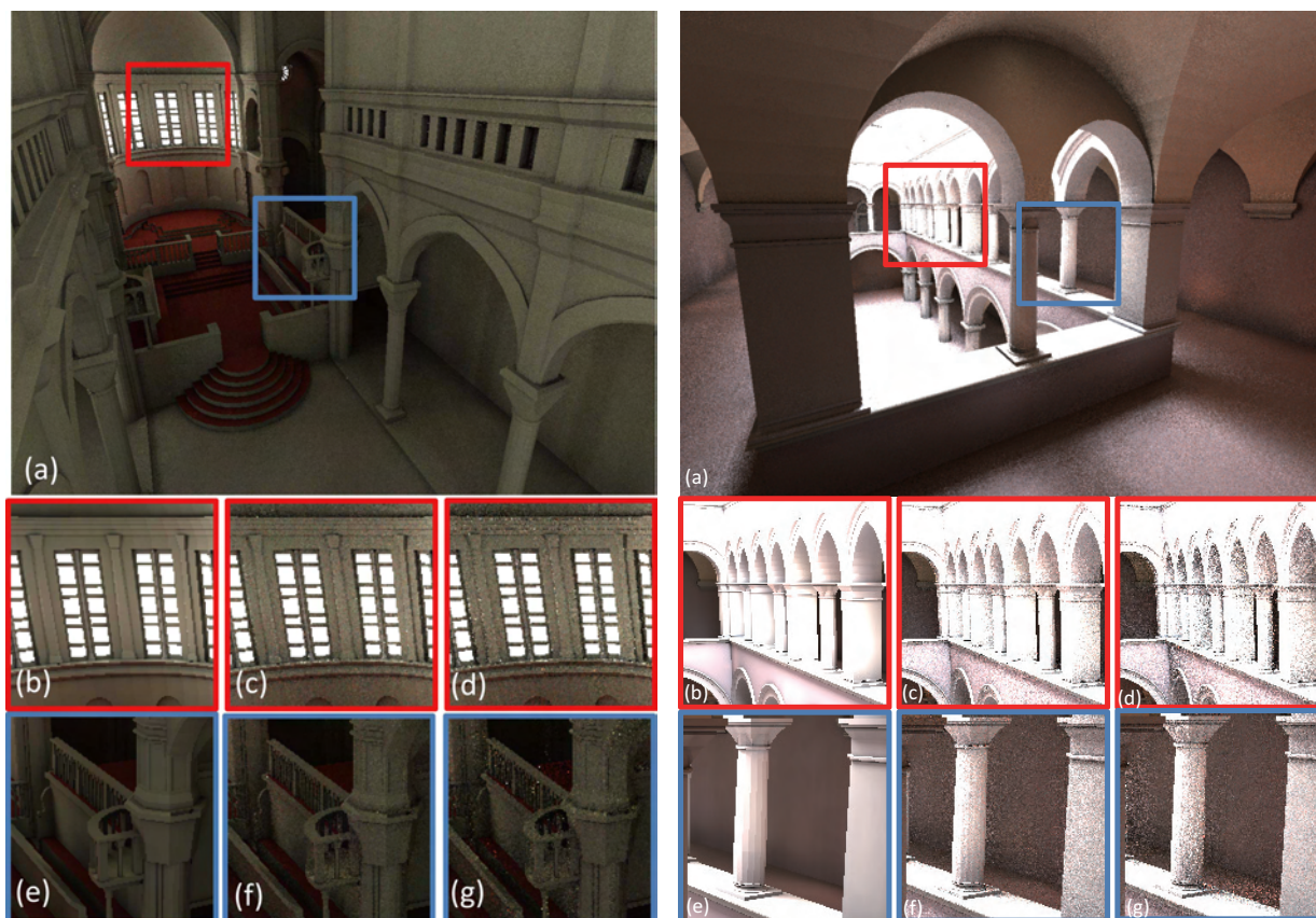
Figure 4: Sibenik scene. (a) rendering result of our method. (b)(c)(d) close-up images of reference, our method, and importance caching, respectively. (e)(f)(g) close-up images of reference, our method, and importance caching. Our method can render less noisy image in equal time rendering compared to importance caching.
