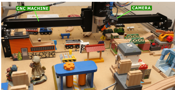
Figure 6: Experimental setup showing a camera mounted on a CNC machine allowing us to capture ground truth information.
