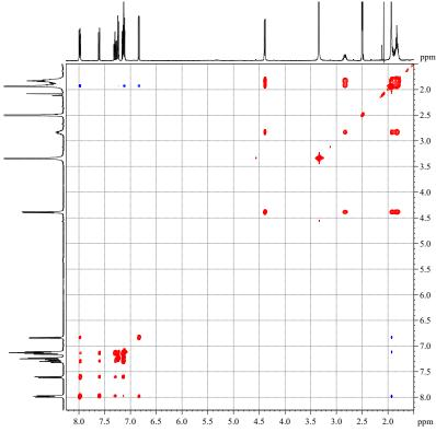
Bruker AVANCE NEO 400, CryoProbe Prodigy; solvent: DMSO- $d_6$
