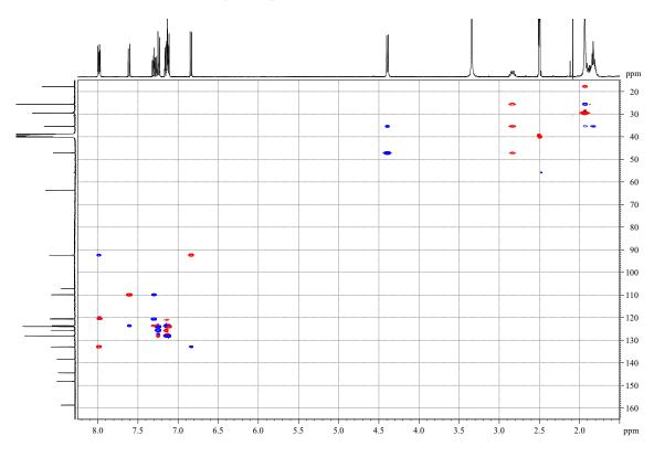
Bruker AVANCE NEO 400, CryoProbe Prodigy; solvent: DMSO-d $_6$
