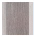
**#4 WELD FINISH** Normally used with #4 material finish when sanitary product contact surfaces are required. 35 Ra target. Request 32 Ra maximum to comply with 3-A standards.
