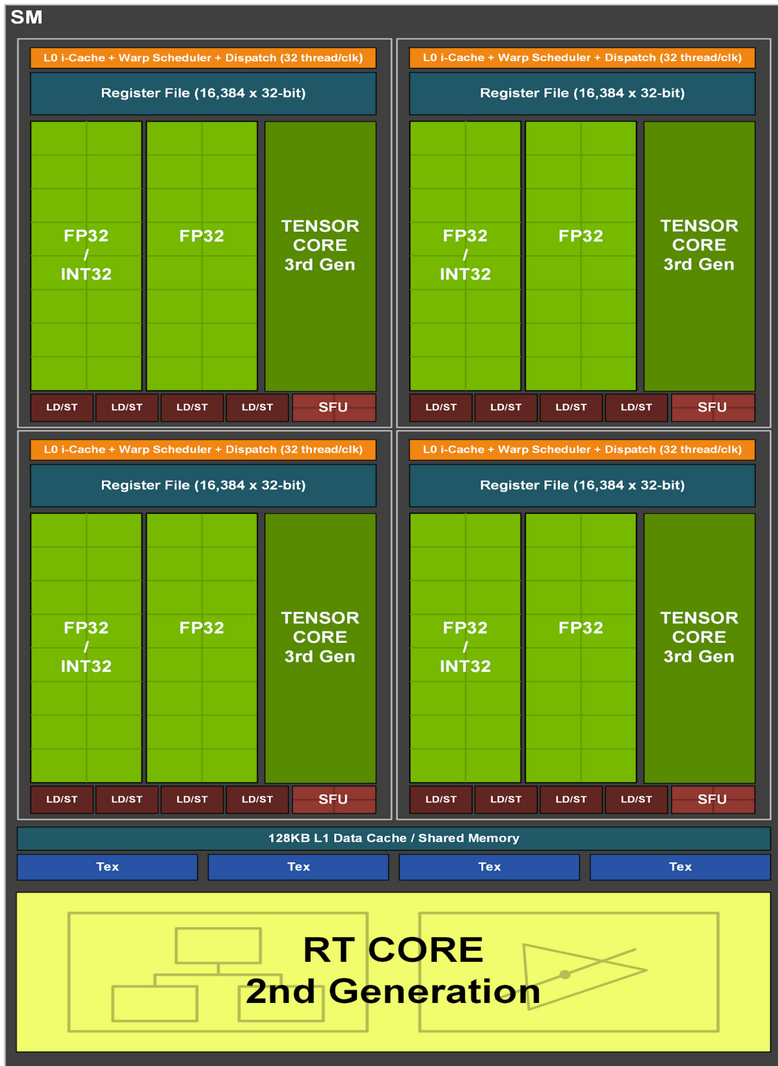
Figure 3. GA10x Streaming Multiprocessor (SM)
