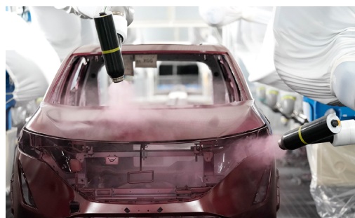
Simultaneous Painting of Body and Bumpers CO 2 emissions have been reduced by simultaneously painting the body and bumpers using a new technology and consolidating them into one process (right) and drying at a low temperature (85°C) instead of the conventional two-step process (left).
