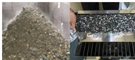
Research on optimization of ASR recovered resin recycling process. Left photo is ASR and right photo is resin recovered from ASR.
