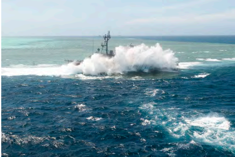
Figure 1-4. Strong wind and surf throughout the winter monsoon season at times restricted the salvors ability to access the vessel and weakened the hull's structure.
