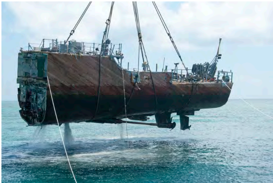
Figure 5-17. Stern section lift, conducted on 30 March, cleared the reef for a final cleanup.
