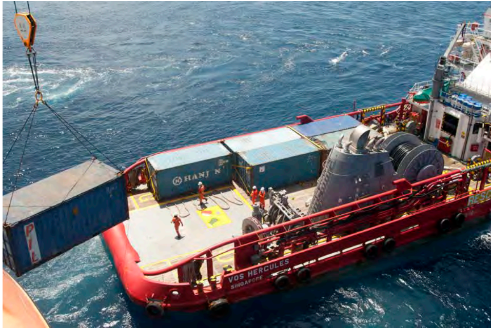
Figure 6-1. VOS Hercules receiving CONEX boxes from SMIT Borneo. Note cable reel and stack already loaded.
