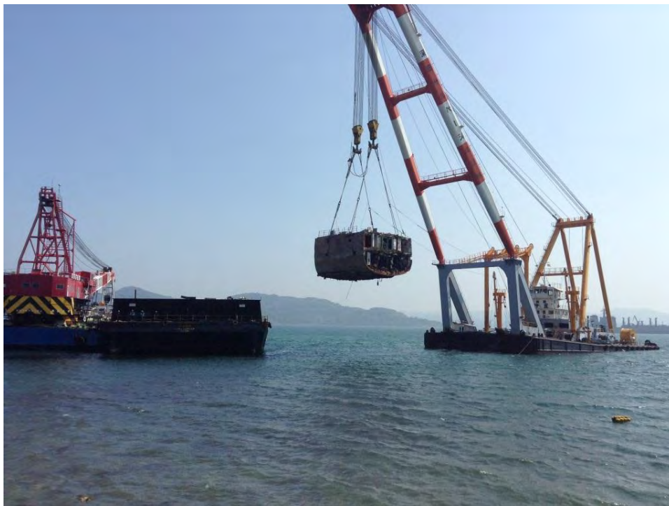
Figure 6-5. GUARDIAN sections being offloaded in Sasebo, Japan.
