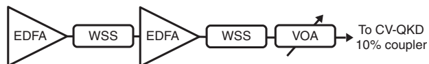
Fig. 8 Noise loading setup. Outline of the experimental setup for generating in-band amplified spontaneous emission (ASE) noise. The wavelength selective switches (WSSs) are generating a wideband notch with 19 dB attenuation (not using the full attenuation as in the transmission experiments). The power is measured on each side of the notch, using an optical spectrum analyzer, and averaged. By knowing the notch attenuation we can calculate the in-band ASE noise power. EDFA Erbium doped fiber amplifier, WSS wavelength selective switch, VOA Variable optical attenuator, CV-QKD continuous variable quantum key distribution
