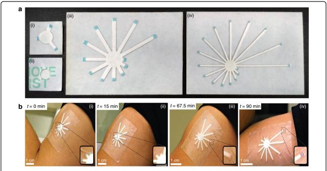
Fig. 3 Prototypes and usage. a Fabricated prototypes of each of the three designs corresponding to the three use cases (i) office person (front side), (ii) office person (back), (iii) half marathon runner, and (iv) ultramarathon runner. b The sweat patch being used on the upper arm of a person working out in the gym showing the sequentially changing color of the tips from blue to red as a function of exercise time (i)—(iv)
