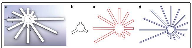
**Fig. 2 Patch parameters and examples of customization. a** Schematic of the patch showing various geometrical design parameters. Comparative geometric designs for three use cases: **b** office work, **c** half marathon, and **d** ultramarathon
