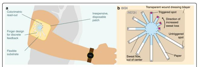
Fig. 1 Device concept. a A wearable device/patch for measuring sweat rate and hydration status. b Conceptual illustration of the hydration monitoring patch with discretized levels of collected sweat which change color when fully wet for easy visibility
