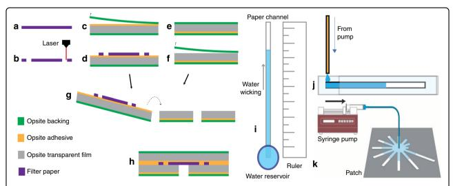
Fig. 6 Patch fabrication process and characterization. a, b Laser machine filter paper, c, d expose adhesive of one polyurethane film and attach the paper, e, f Laser machine wicking port on another piece of film and remove the top backing, g, h stack together films for assembly. Remove backings before use. Test setup for material wicking speed characterization: i unlimited-source wicking, j flow-limited wicking. k Patch characterization setup using a syringe pump
