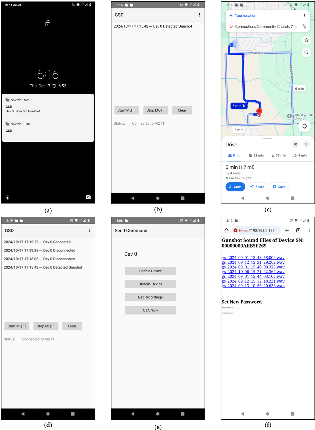
Figure 12. Screenshots of the smartphone app showing: (a) gunshot event notification; (b) event log with timestamp; (c) navigation direction on the gunshot location using Google Maps; (d) device connection status log; (e) command buttons to control device; (f) accessing gunshot sounds stored on the device.
