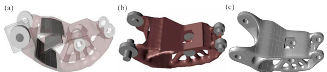
Figure 5. Manual reconstruction: (a) Model package; (b) Opening of fixed holes; and (c) Reconstruction effect.
