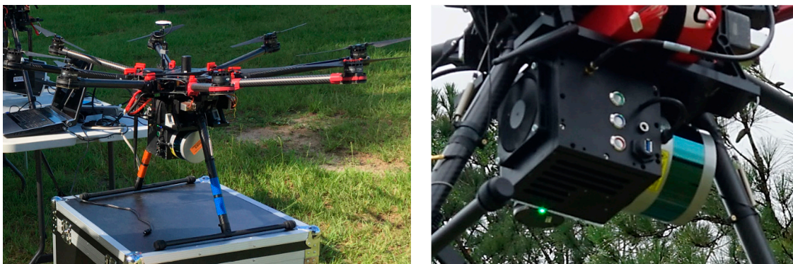
Figure 1. The unoccupied aerial systems (UAS) laser scanning system used in the study.
