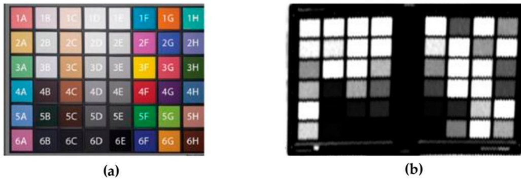
Figure 7. (a) A photograph of a colored test field (DatacolorSpyder CHECKER). (b) Scan (intensity) of the test field in grayscale (0–255) [62].
