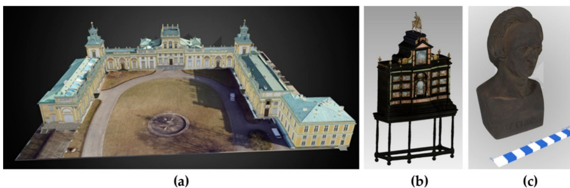
Figure 18. (a) The 3D model of the Palace and Markoniówka based on the integration of photogrammetry and TLS data, (b) the 3D model of the King Jan's cabinet, (c) the 3D model of the bust of Frédéric Chopin (Museum of King Jan III's Palace at Wilanów).
