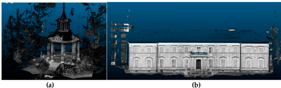
Figure 15. TLS point clouds acquired for the (a) Chinese Gazebo and (b) one of the Palace elevations (Museum of King Jan III's Palace at Wilanów).
