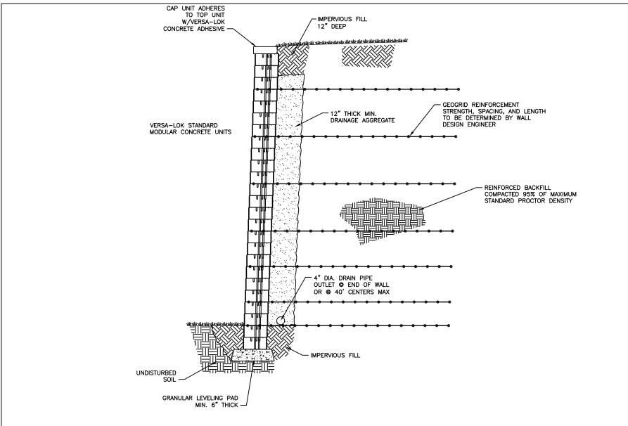
TYPICAL SECTION REINFORCED RETAINING WALL
