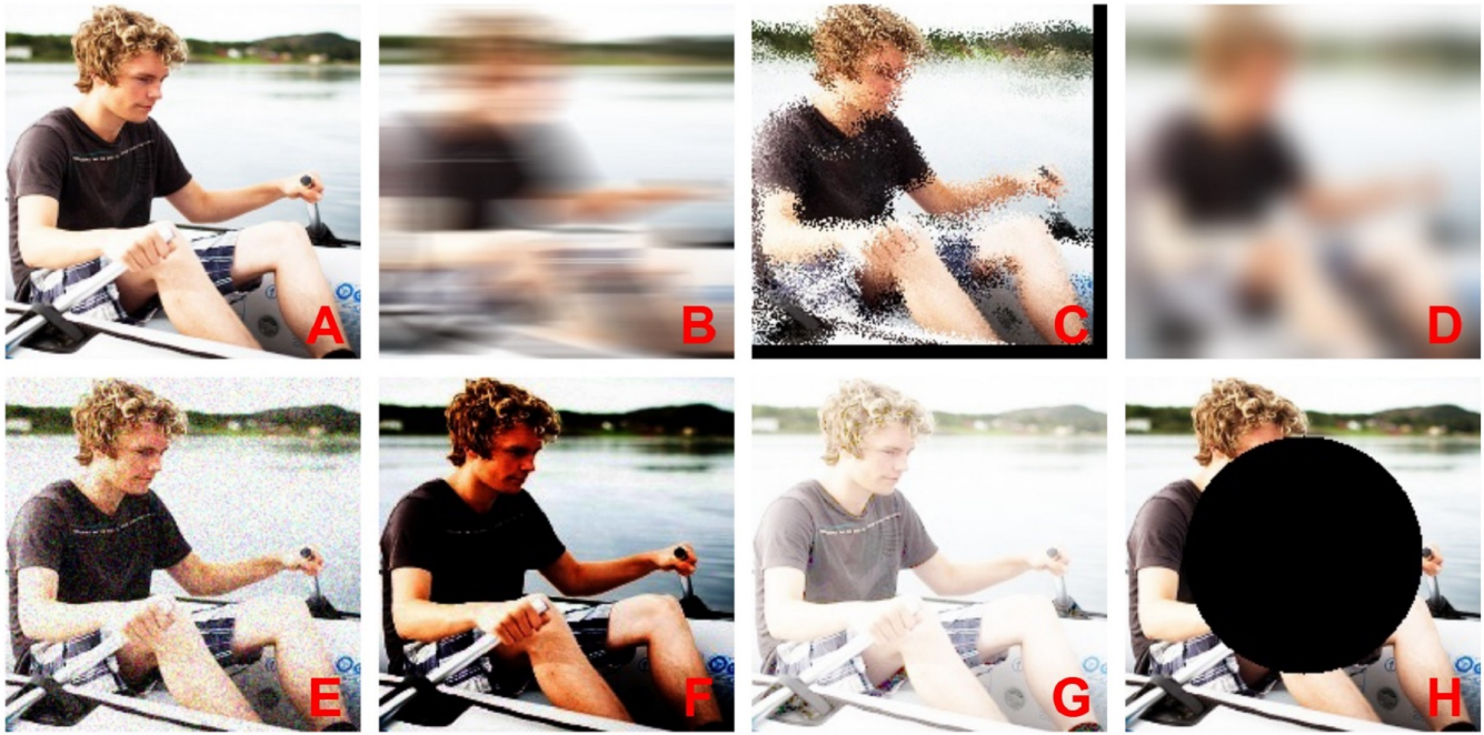
Figure 3: Effects of environmental factors on the input image (Taken from (Bakhshi Germi, Rahtu, and Huttunen 2021)): (A) Original image, (B) Movement of camera/object (Motion blur), (C) Raindrop on the lens (Frosted-glass blur), (D) Out-of-focus object (Gaussian blur), (E) Low illumination (Gaussian noise), (F,G) Improper balance of light and darkness (Low/High brightness), and (H) Obscured object (Occlusion).
