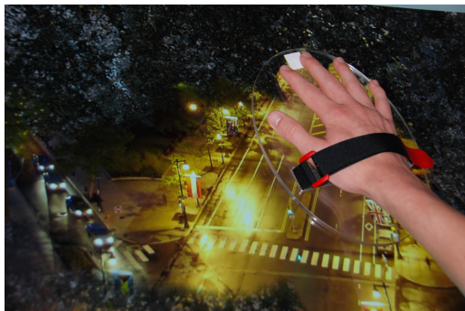
Figure 5: The module “Window Washing” with physical cleaning element fixed to the user’s hand.
