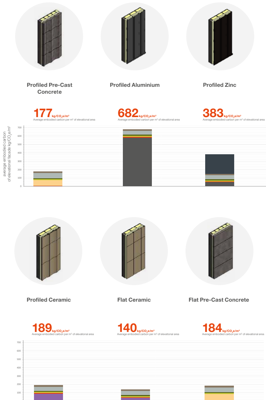
Figure A.6.3.1 – Embodied carbon study of facade design options at stage 2. Data and images courtesy of Hawkins\Brown Architects LLP, not to be copied or reproduced without consent. Results assessed by H\B:ERT tool covering stages A1-A5, B4 and C1-C4 according to BS EN 15978:2011.
