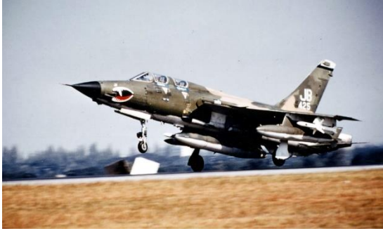
Figure 3 - A USAF F-105G Thunderchief aircraft, armed with AGM-45 and AGM-78 anti-radiation missiles.
