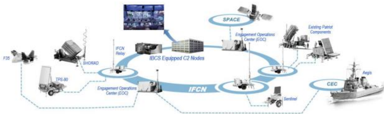
Figure 1 IBCS Integrated Fire Control Network connects sensors, weapons and C2 Nodes to include bridging with other Fire Control Networks Such As CEC
