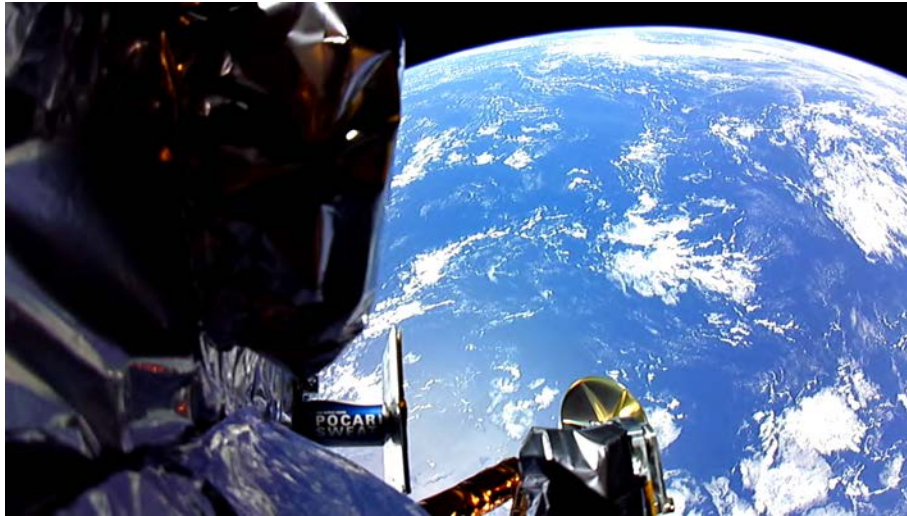
FIGURE 3: This image was taken by camera 1 moments after successful separation from United Launch Alliance's Vulcan rocket. Counterclockwise from top left center is the DHL MoonBox, Astroscale's Pocari Sweat Lunar Dream Time Capsule, and a Peregrine landing leg. In the background is our big blue marble, our home planet, Earth.
