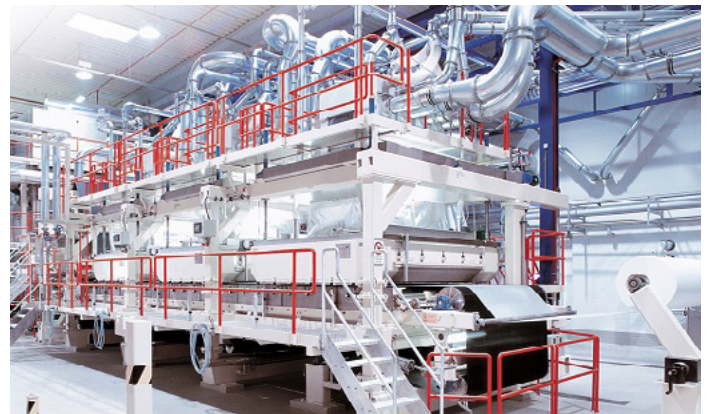
Nonwovens production line that can manufacture feminine hygiene products, diapers, wet wipes, food pads and tabletop items among other products. Credit: Oerlikon Neumag Airlaid Technology
