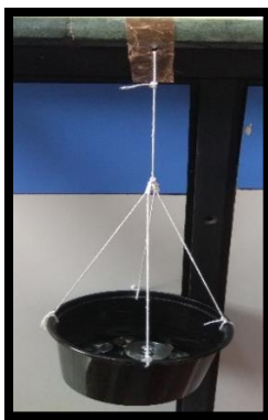
Fig. 2. Strength test of coir bioplastic
