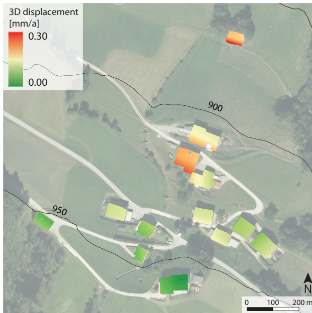
Figure 9. Derived 3D displacement vectors derived from the laser scanning data showing deformation of extracted roofs in the area affected by the active landslide.
