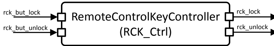
Figure 3.15.: Interface Specification of the Standard RemoteControlKeyController Component
