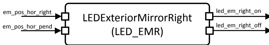
Figure 3.35.: Interface Specification of the LEDExteriorMirrorRight Component
