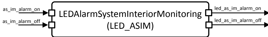
Figure 3.41.: Interface Specification of the LEDAlarmSystemInteriorMonitoring Component
