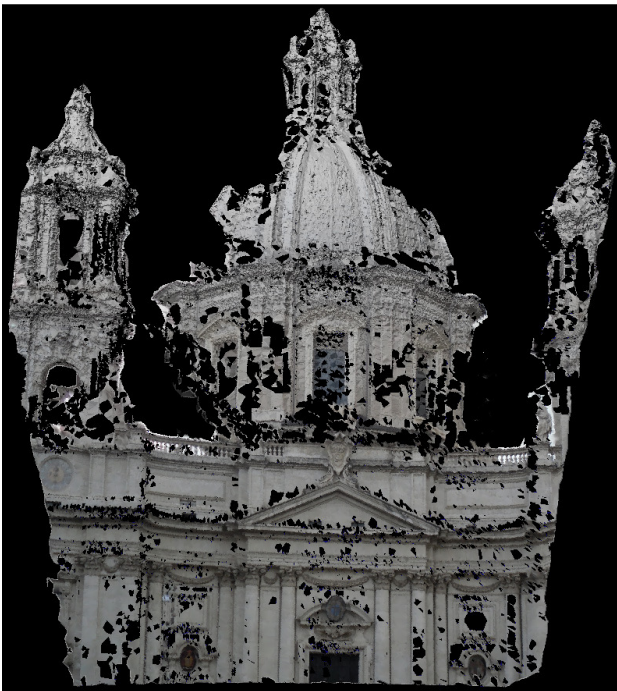
Figure 7. Orientation of Piazza Navona sequence. Top : camera stations and tie points. Bottom : DSM of the façade church of Sant'Agnese.
