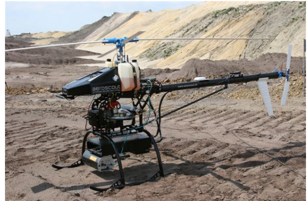
Figure 2: Picture of the Scout BI-100 UAV helicopter during airborne 3D laser flight testing in Germany. For these tests a RIEGL laser scanner LMS Q160, an onboard computer system, a broadband data link, and a DGPS system with a total payload weight of approx. 15 kg have been attached to the helicopter. The average flight endurance with 10 l of fuel is 1.5 h.
