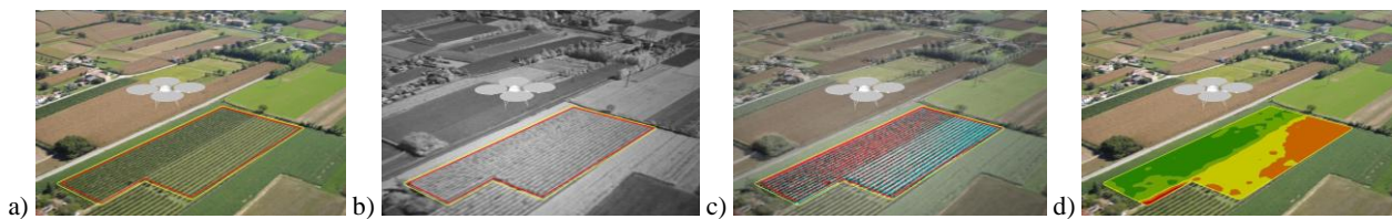
Figure 7: The studied wine yard area (a), seen in the NIR domain (b), with false colors (c) and the estimated NDVI index (d).
