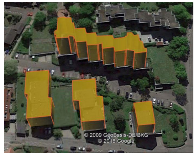
Figure 9- google earth view of LoD2 CityGML model created by open source software
