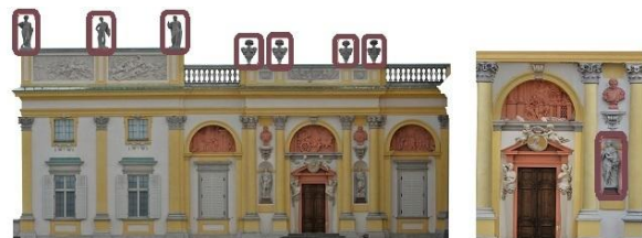
Figure 3 Fragments of orthoimages of the historical facade from TLS with marked elements acquired from the image matching process.
