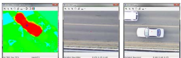
Figure 11. The blunder due to moving object (Left: DSM, Centre: left image, Right: right image)
