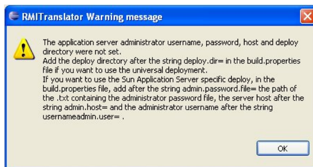
Figure 48. Warning message at the end of the RMI to Webservice transformation process due to the missing application server deploy directory or one between the application server username, password or host fields.
