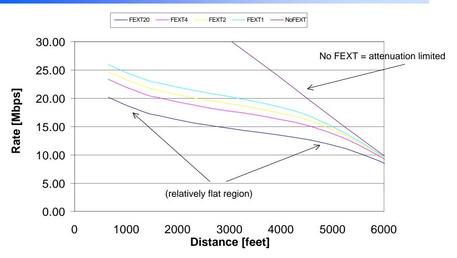
Results for arbitrary 24AWG distribution cable, 2MHz carrier - for illustration only
