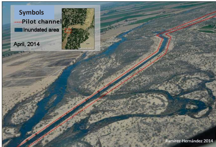
Figure 2-5. Oblique aerial view of a typical portion of Sector 4 during the pulse flow, showing the extent of inundation of the pilot channel and off-channel depressions.
